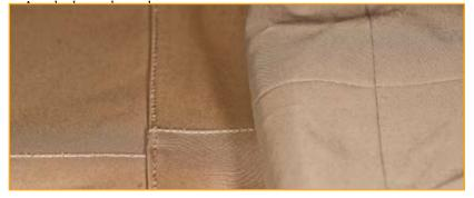
Sonic weld vs sewn seam for waders. Leg seam from SonicSeam waders (right) and a standard wader with a sewn seam. The Sonic Weld is cleaner and lighter and gives a wader less bulk and more flexibility
